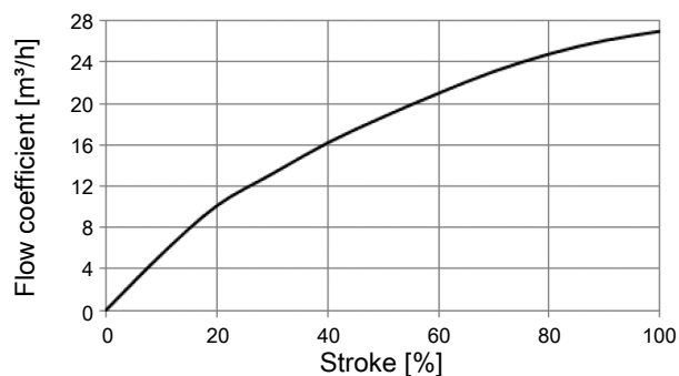
Fig. 23: Flow characteristics seat size 32, actuator size N (ø90)
