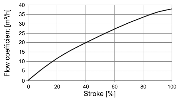
Fig. 25: Flow characteristics seat size 40, actuator size N (ø90)
