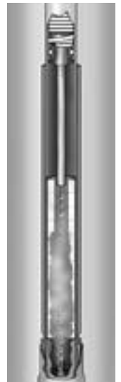
Vapor quenches arc at first current zero
