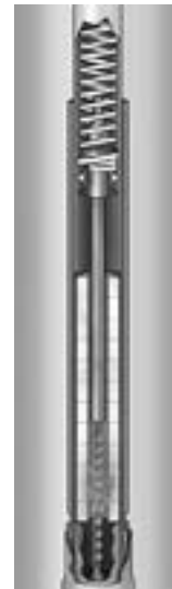
Rod withdraws elongating arc and vaporizing boric acid
