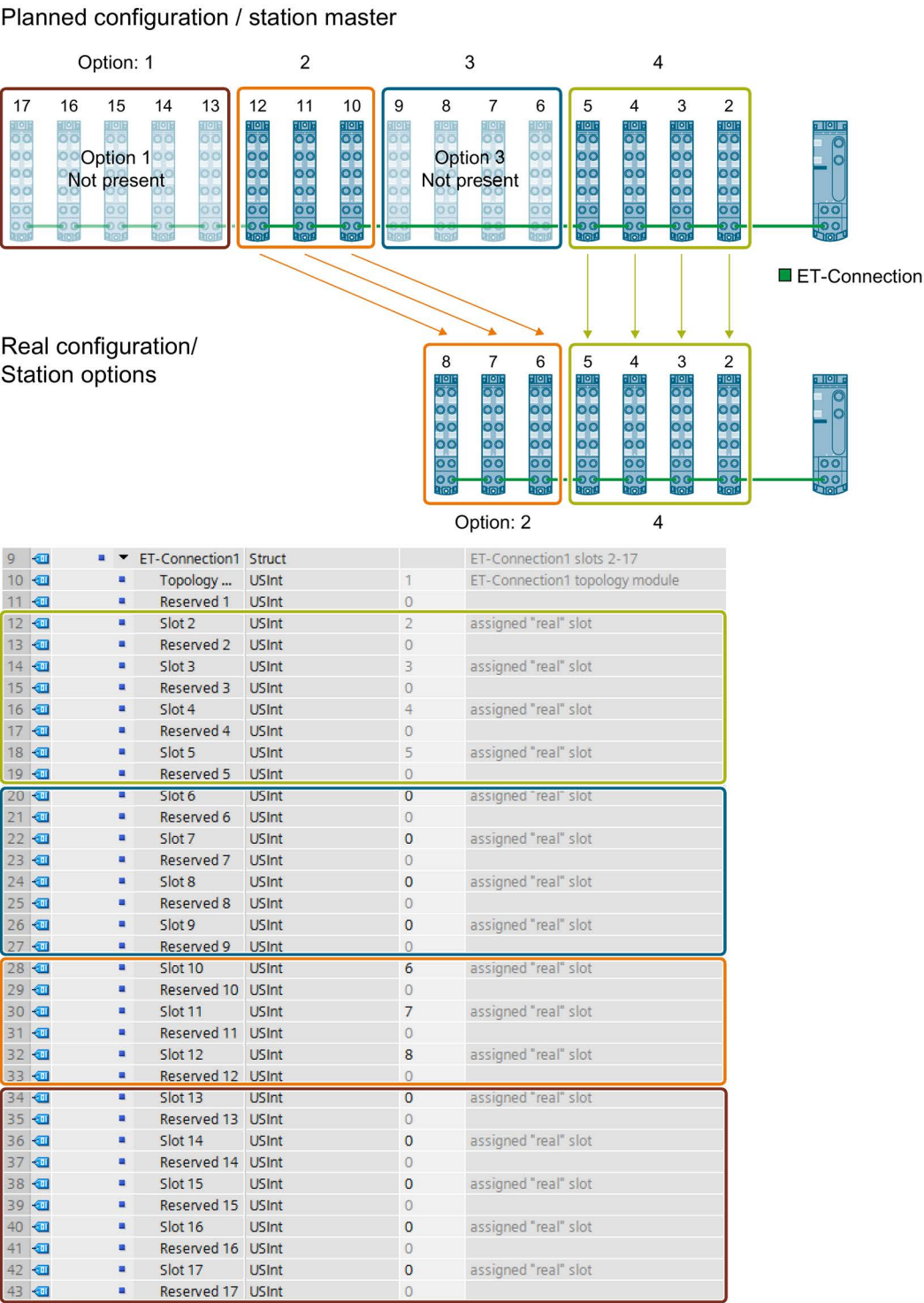
Figure 7-6 Example: Hardware configuration of Station option 2 and 4 with the associated control data record in STEP 7
