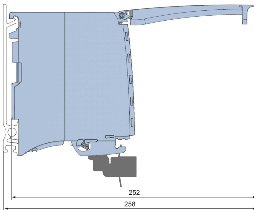
Figure A-2 Dimension drawing of the AQ 4xU/I HF module, side view with open front cover
