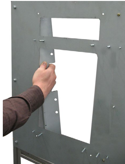
Locate the reinforcement plate on the mounting panel.
