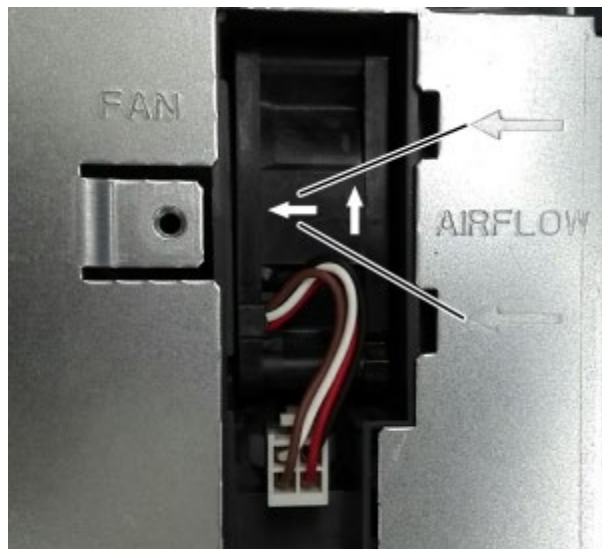
Figure 13-1 Arrows on the fan for the air flow direction
