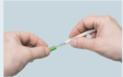
Remove the outer sheath and expose the braided shield
