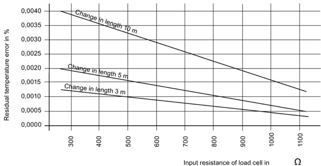
Figure 4-1 Residual temperature error for a load cell per 10 K temperature change when shortening or lengthening the connecting cable
