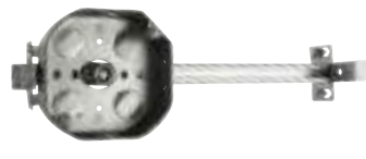
54151 J 1/2 Mounted on 6010-DW bar adjustable 10 1/2" to 18 1/2". Offset for 1/2", 3/4" or 7/8" plaster. Maximum horizontal positioning. 3/8" fixture stud.
