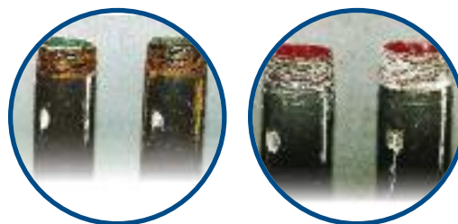
Examples of Spray-Galvanized (Hot-Galvanized) Threads after 42-day salt-fog test
